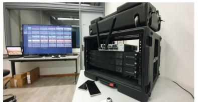
Patras 5G Autonomous Edge, is a mobile box, containing everything from the 5G New Radio and 5G Core, Network and Service Orchestrations including a Virtualized environment based on OpenStack technology. <a href="http://wiki.patras5g.eu/5g-autonomous-edge">http://wiki.patras5g.eu/5g-autonomous-edge</a>
