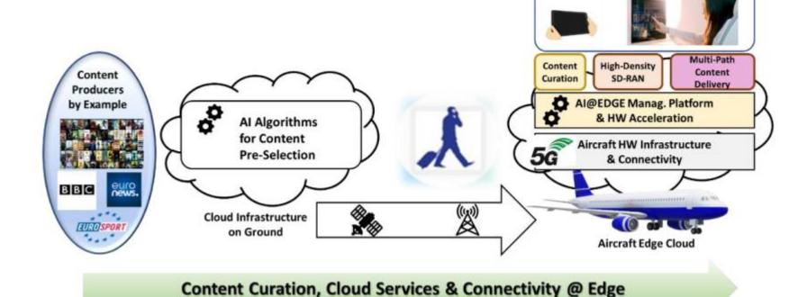
→ With the rise of 5G and network softwarization, the cabin infrastructure, composed of servers, wireless termination points and seat embedded screens, has the potential to transform itself into a full edge cloud.
