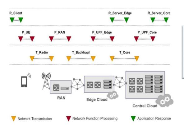
The <u>End-to-End Latency</u> here is considered to be composed of three types of delay, that is:
